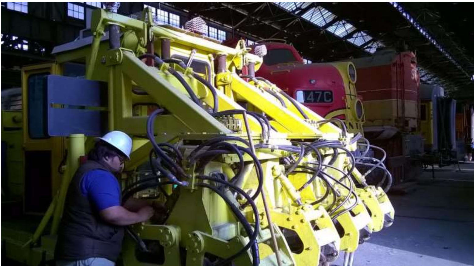
Anthony greases the many moving parts on the tamper's work-head
