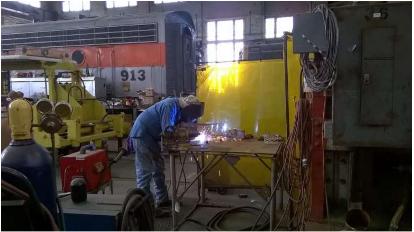
Cliff builds a protective shield for the Jackson 125's new air-horn
