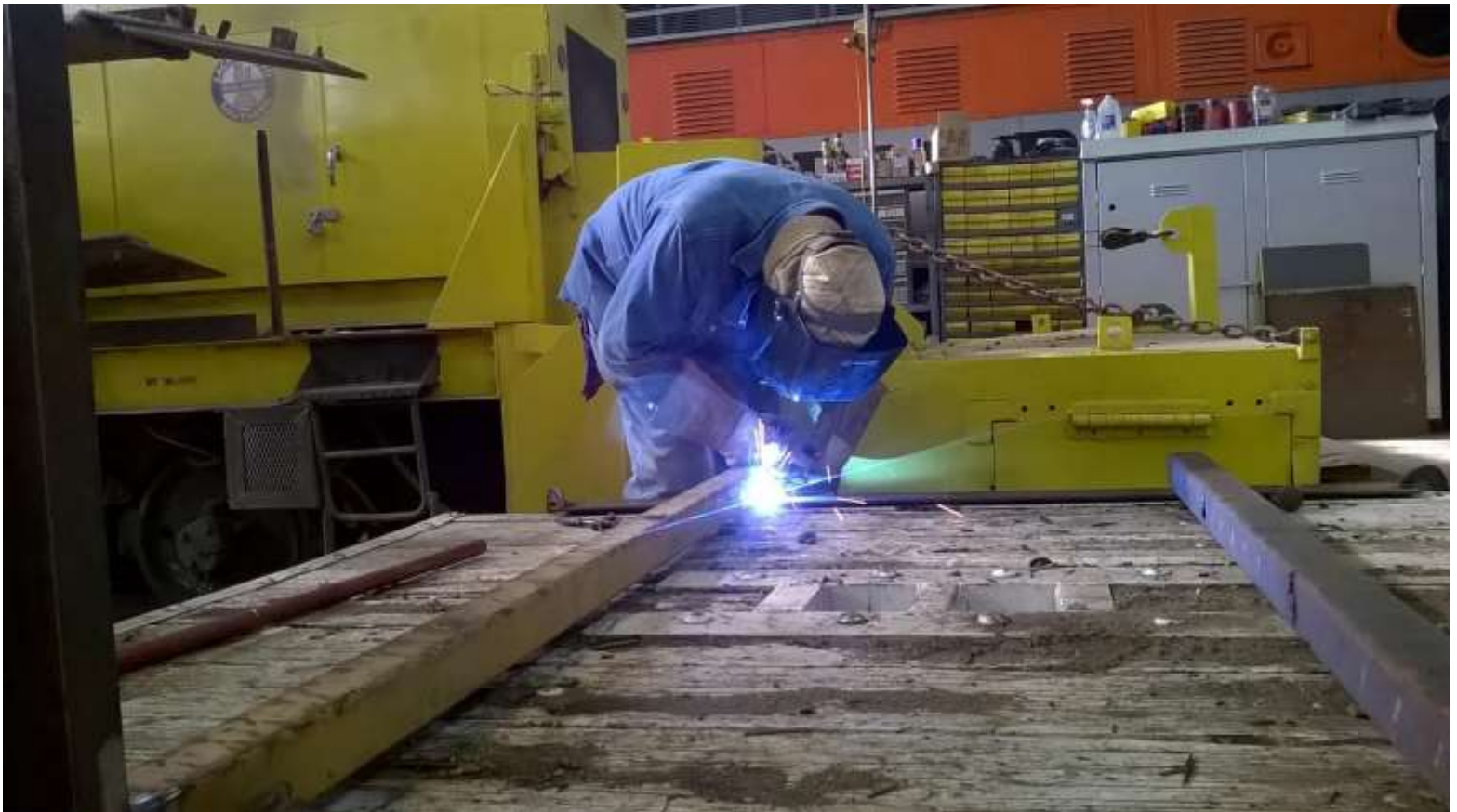
Cliff welds components for the new railings being added to a MOW flatcar
