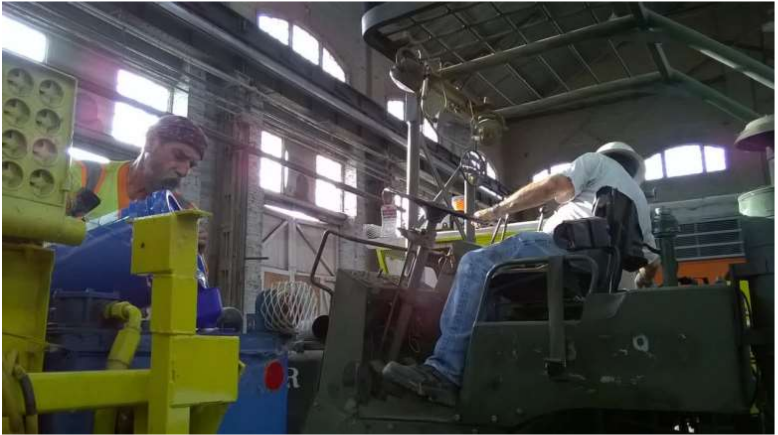
Next, Joe adds hydraulic fluid to the tamper as Mike H. moves Big Green to provide easier access for working on the engine
